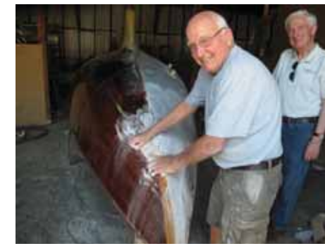
Mike Pongracic faring the epoxy coating on the hull, with Bill West looking on.
